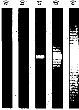
Fig. 2. Images of single slit diffraction patterns taken at increasing exposure times: (a) 1/4000, (b) 1/250, (c) 1/15, (d) 1, and (e) 15 s.
