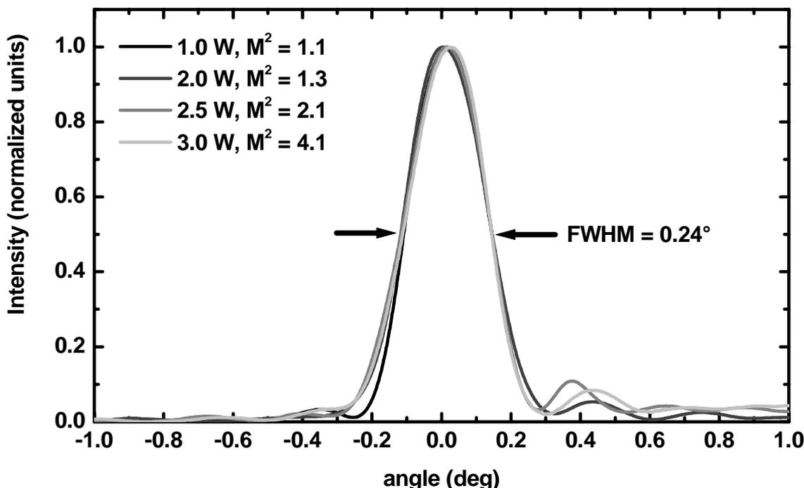
Figure 4: Dependence of the lateral far field profiles of tapered high-power diode lasers ( $L_1 = 500 \mu\text{m}$ ,  $L_2 = 2500 \mu\text{m}$ ) on the output power after removal of the quadratic phase curvature by a cylindrical lens at a heat sink temperature of 20 °C (cw). Additionally the measured values of  $M^2$  are given corresponding to the output power.
