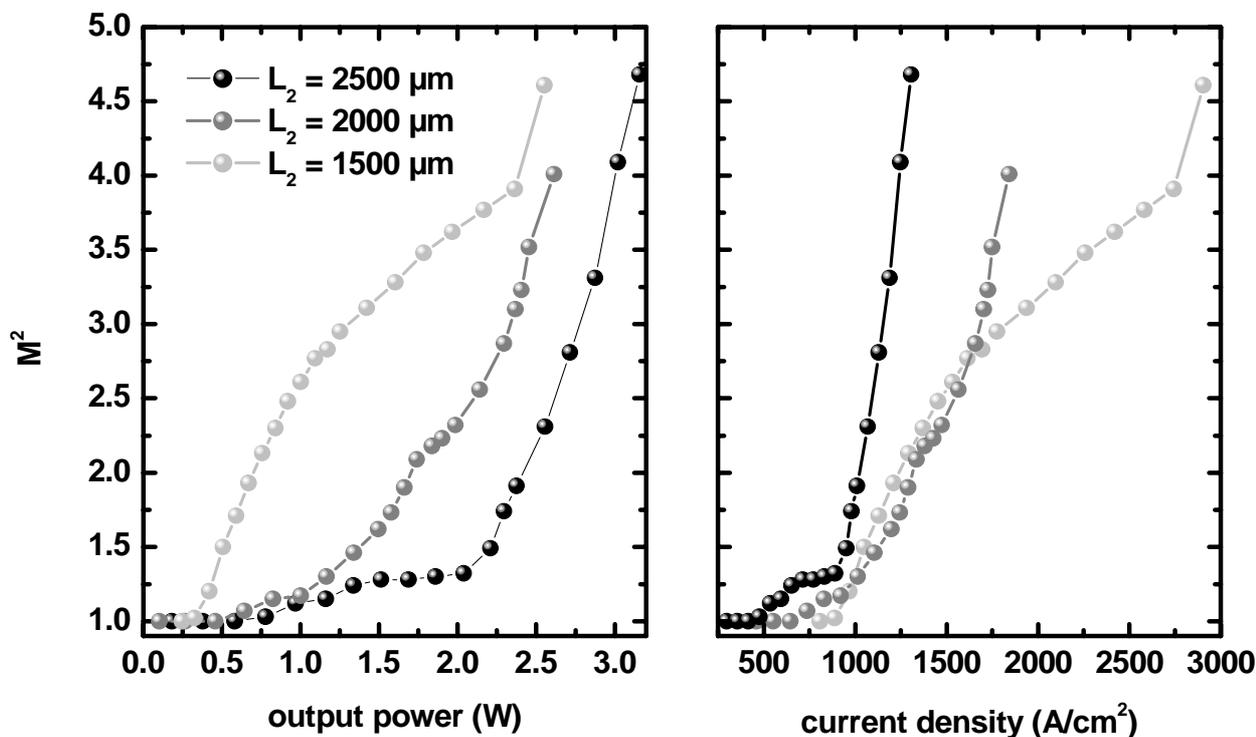
Figure 3: Dependence of the beam quality parameter  $M^2$  on the output power and the current density for different lengths of the tapered section  $L_2$  at a heat sink temperature of 20 °C (cw).
