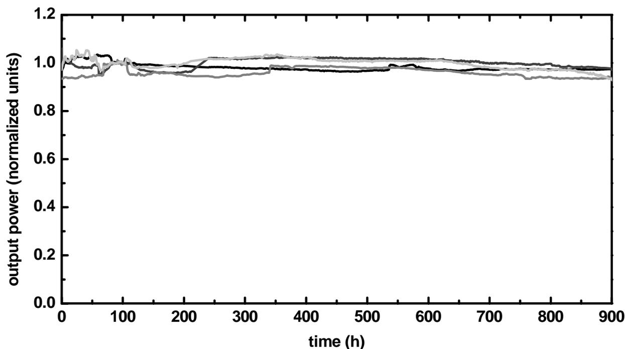
Fig. 5: Reliability test of tapered high power lasers ( $L_1 = 500 \mu\text{m}$ ,  $L_2 = 2500 \mu\text{m}$ ) at an output power of 1.8 W and a heat sink temperature of 50 °C. Assuming an activation energy of 0.35 eV, a lifetime of more than 7,500 h can be deduced from these data.
