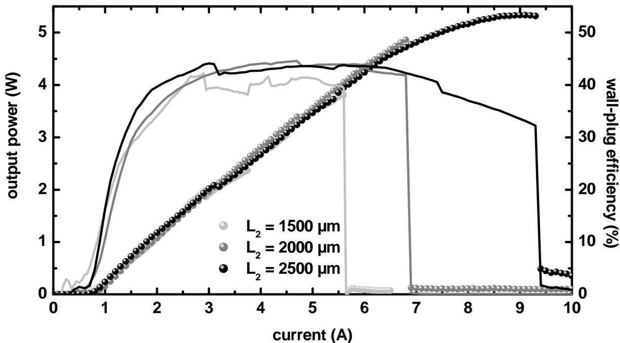
Figure 2: Typical current-power characteristics (dots) and the wall-plug efficiencies (lines) of tapered diode lasers with different lengths of the tapered section at a heat sink temperature of  $20\ ^\circ\text{C}$  measured in continuous wave mode.
