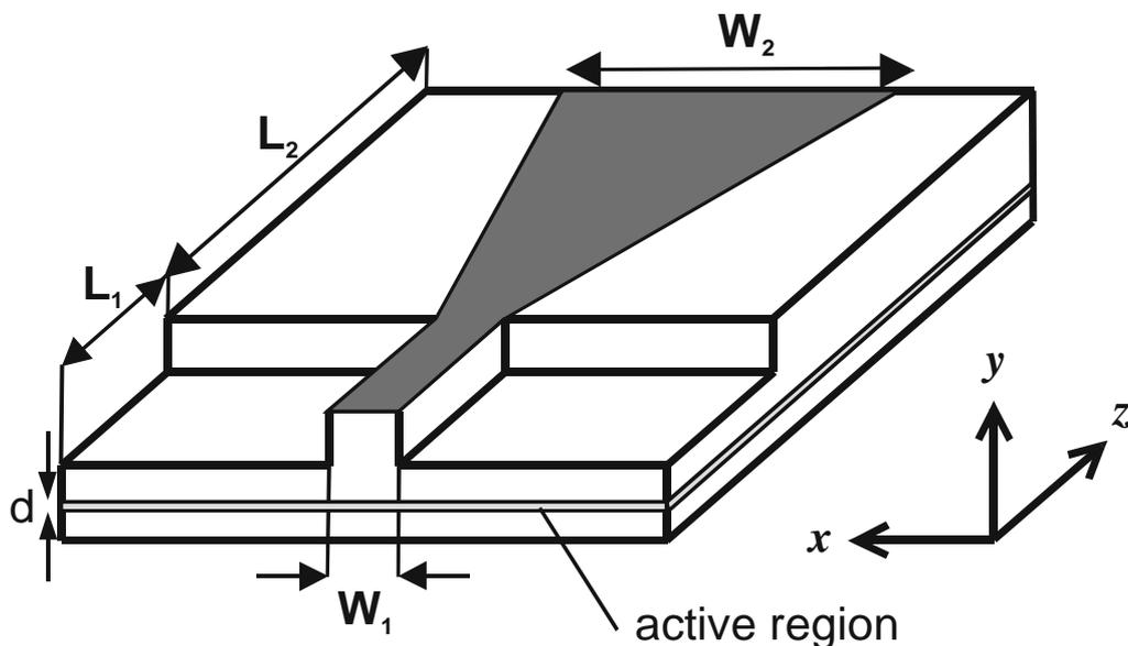
Figure 1: Schematic of a tapered diode lasers with a ridge waveguide for mode filtering. The length of the ridge section  $L_1$  varies between 100  $\mu\text{m}$  and 500  $\mu\text{m}$ , whereas the length of the tapered section varies between 1500  $\mu\text{m}$  and 2500  $\mu\text{m}$ . The tapered angle is  $6^\circ$ .
