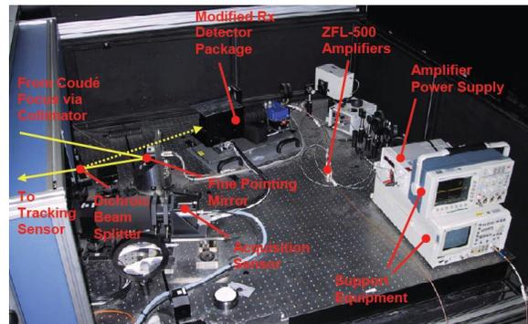
Figure 10: RDP at the OGS Optical Bench
