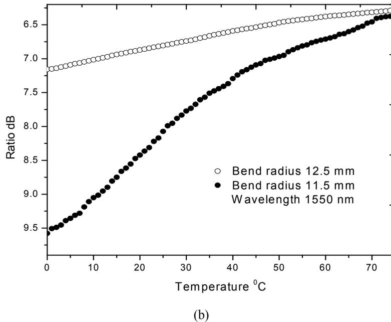
Fig 3. (a) Comparison of temperature response of the macro-bend fiber with different absorption coatings (b) Temperature response of the sensor coated with Indian ink for two different bend radii
