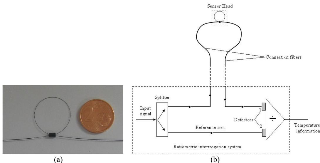
Fig 1. (a) The sensor head (b) Schematic of the macro-bend fiber temperature sensor system
