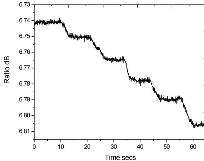
Fig 4. Variation in ratio for a step change of temperature of 1 °C from 30 °C to 25 °C
