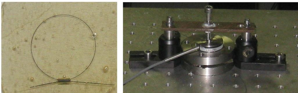
Fig 6. (a) Sensor embedded in epoxy (b) Experimental arrangement to study the effect of stress
