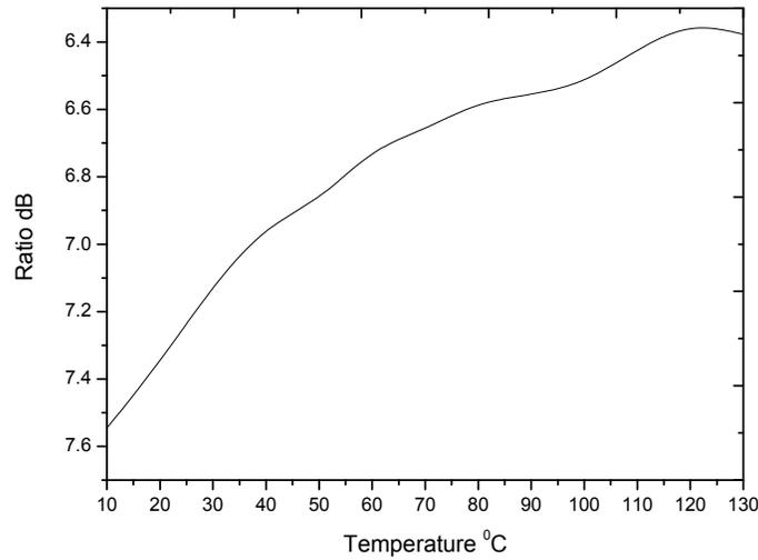
Fig 5. Temperature response of the sensor for a temperature up to 130 °C
