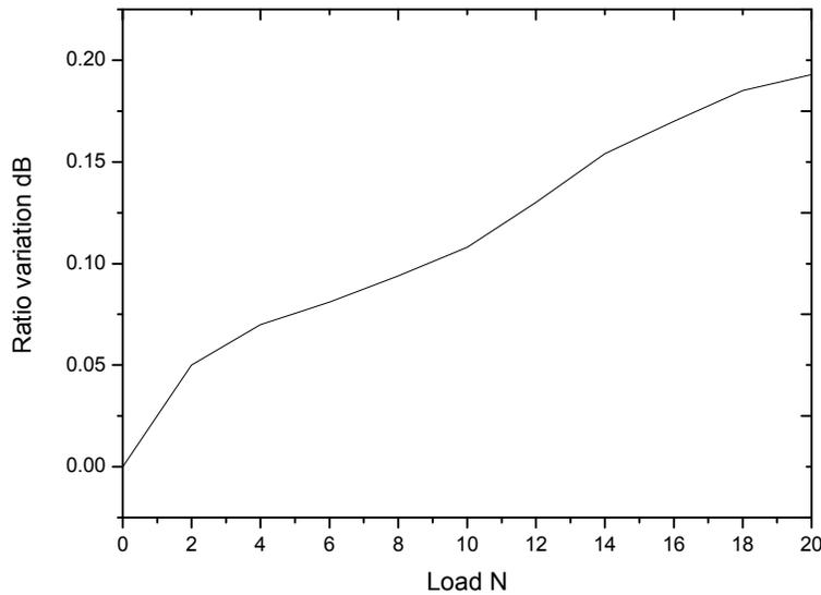
Fig 7. Measured variation in the ratio response of the sensor embedded in an epoxy at 1550 nm when load is applied
