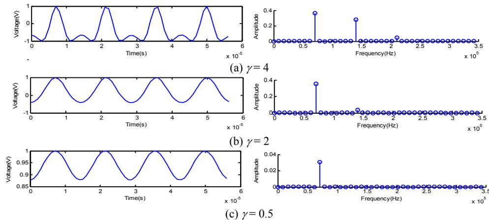
Fig.2. The time domain signals and the frequency domain signals
