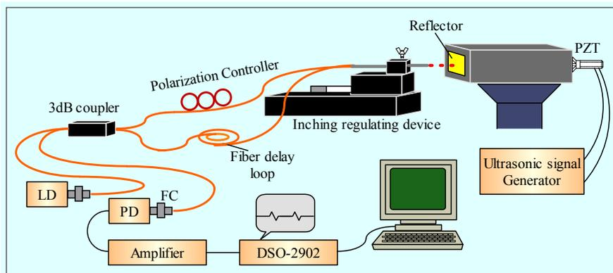
Fig.6. Experimental setup of open-loop Sagnac fiber optical sensor system
