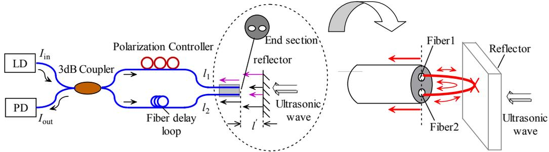
Fig.1. The principle of the open-loop fiber optic sensor
