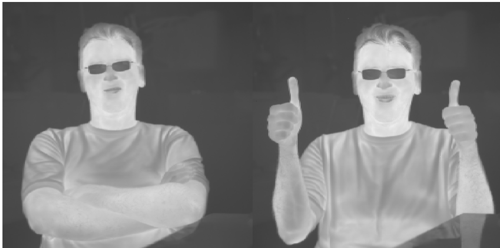
FIGURE 1. Pictures of a student taken with the 1024 \times 1024 FPA at operating temperature of 81K (left) and 68K (right)
