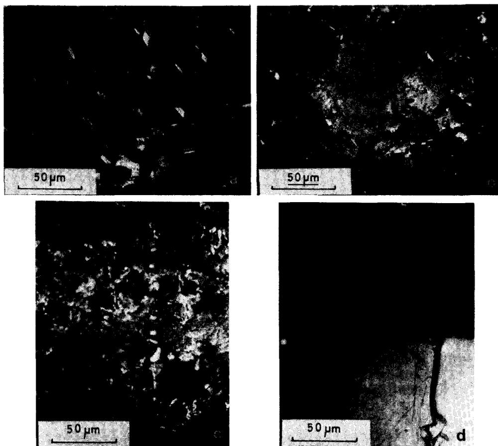
Fig. 2. Optical micrographs of oriented layers of AlSb on (111)GaSb substrates. (a), (b), (c) Different aspects of surface morphologies of layers obtained with experimental conditions reported in table 1. (d) Cleaved section of a 8  $\mu\text{m}$  thick AlSb layer on (111)GaSb substrate.
