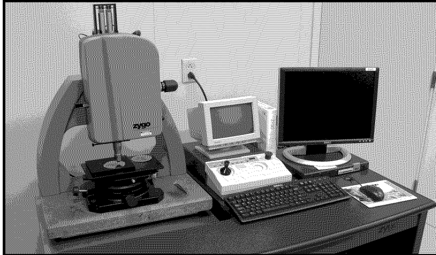
Figure 4-5. Optical profiler used to obtain vertical measurements of fabricated MEMS structures.
