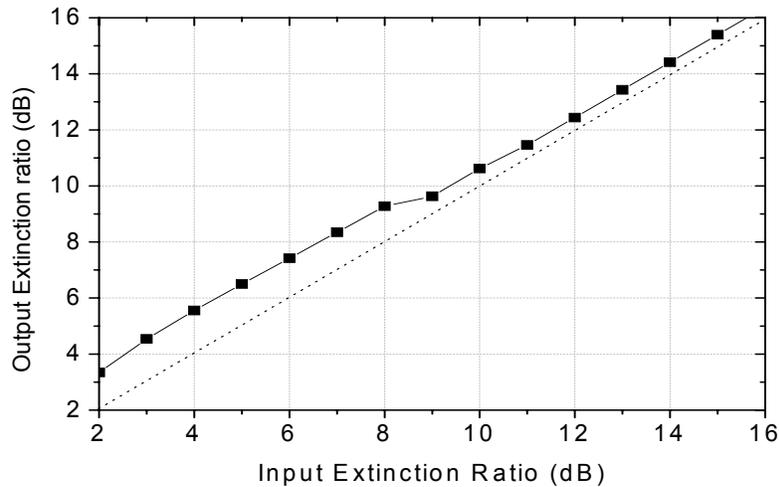
Figure.10. Output Extinction Ratio as a function of the input Extinction Ratio
