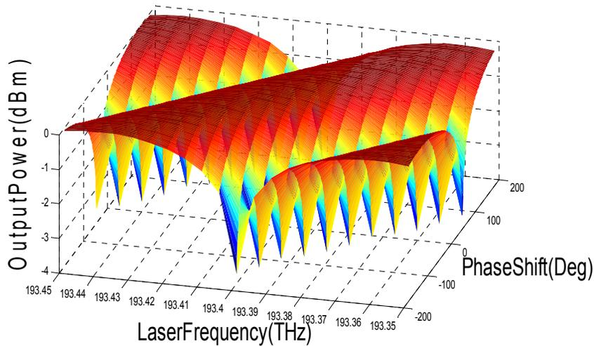
Figure.7. Output power versus both of the change in phase shift of Mach-Zehnder interferometer and laser frequency
