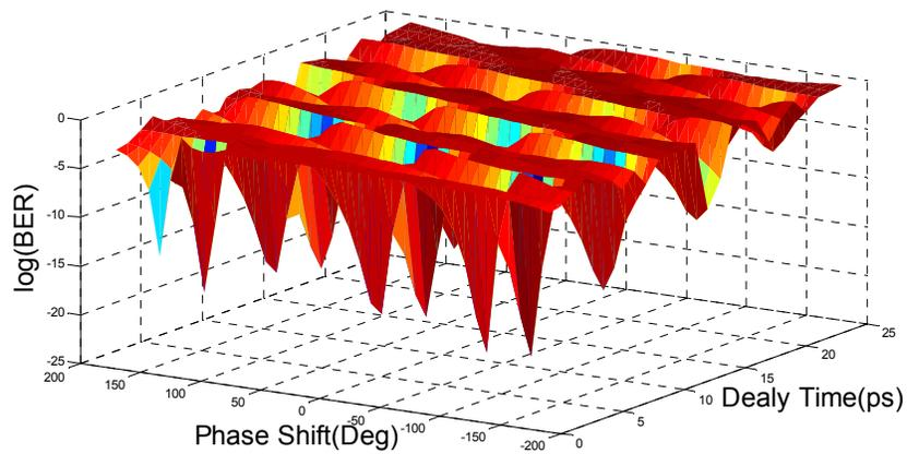
Figure.6. Bit-Error-Rate(BER) versus both of the change in delay time and phase shift of Mach-Zehnder interferometer
