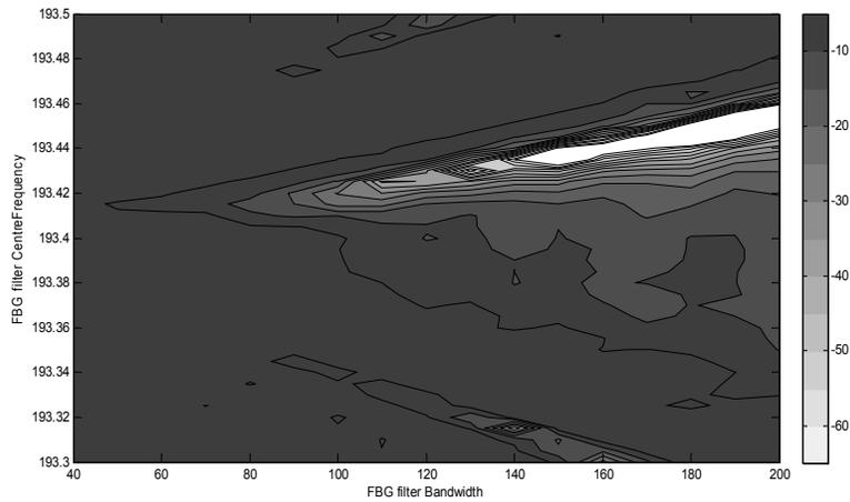
Figure.8. Bit-Error-Rate(BER) versus both of the change in bandwidth and center frequency of Bragg Grating Filter
