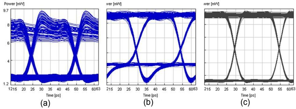
Figure.4. Obtained eye diagrams for the (a) original(distorted) signals(b)signals after Bragg Grating Filter (c)signals after 2R regeneration
