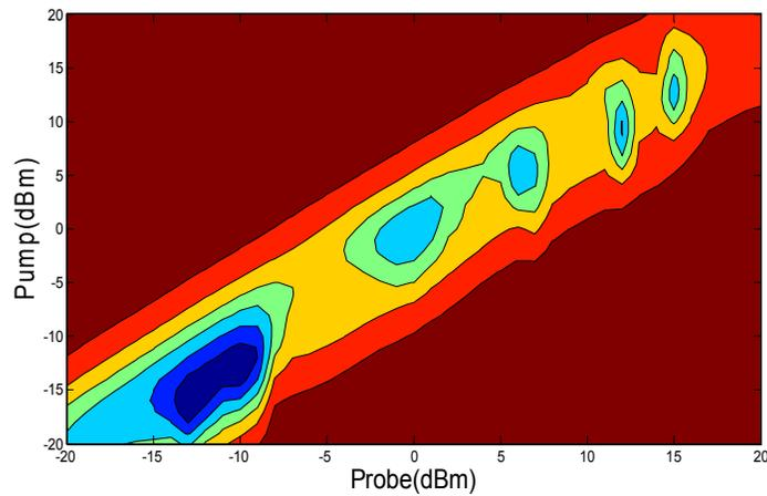
Figure.5. Bit-Error-Rate(BER) versus both of the change in pump light power and probe light power. From Fig.5. , it is obvious that there is a pair of optimal value for pump power and probe power to make BER the lowest. And we find the optimal value for the pump is about -13dBm and for probe -16dBm.
