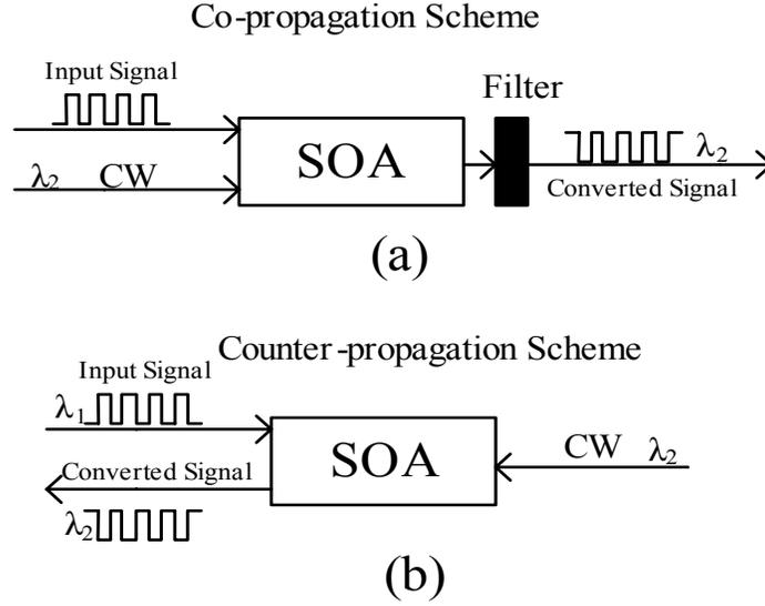
Figure.1. Principle of XGM in SOA
