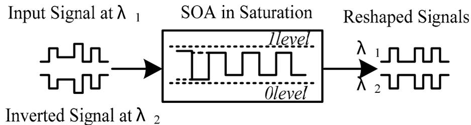
Figure.2. XGC working principle
