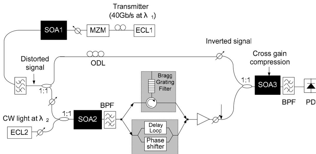
Figure.3. Numerical setup of 40Gb/s 2R Regeneration Based on Cross-Gain Compression in Semiconductor Optical Amplifiers
