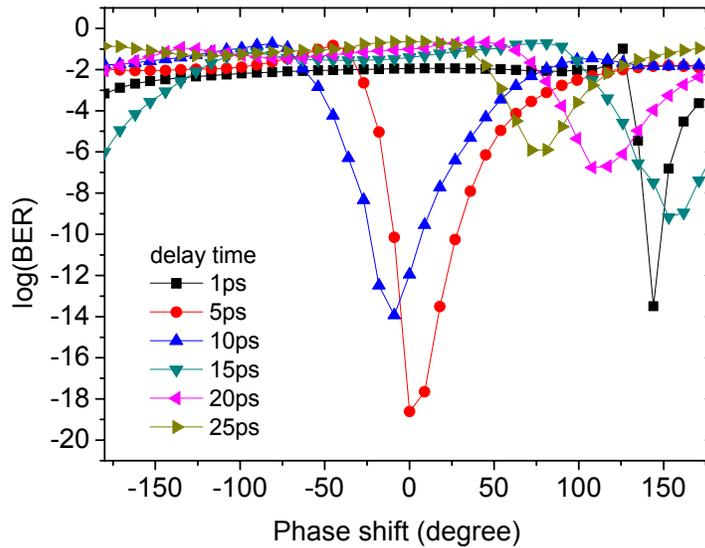
Figure.9. BER versus phase shift with different delay time in Mach-Zehnder interferometer
