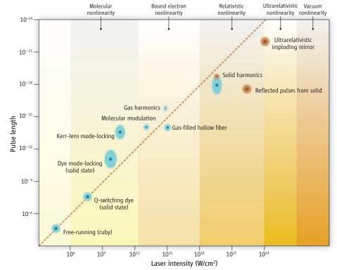
**Shorter, more intense.** An inverse linear dependence exists over 18 orders of magnitude between the pulse duration of coherent light emission and the laser intensity. These entries encompass different underlying physical regimes that exhibit molecular, bound atomic electron, relativistic plasma, ultrarelativistic, and vacuum nonlinearities. Blue patches represent experimental data; red patches denote simulation or theory.
