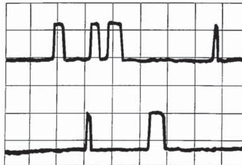
Figure 4. Waveform of burst noise in a reverse-biased (7.5 V) germanium junction. The horizontal scale is 20 ms div -1 and the vertical scale 20 nA div -1 . After Wolf and Holler (1967). © American Institute of Physics. Reproduced with permission.
