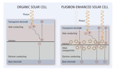
**Better reception.** In an organic solar cell, sunlight frees an electron (–) and an electron vacancy, or hole (+), which migrate to the border between different materials and then to oppositely charged electrodes (*left*). Adding metal nanoparticles (*right*) increases the light absorption and the number of charges generated.
