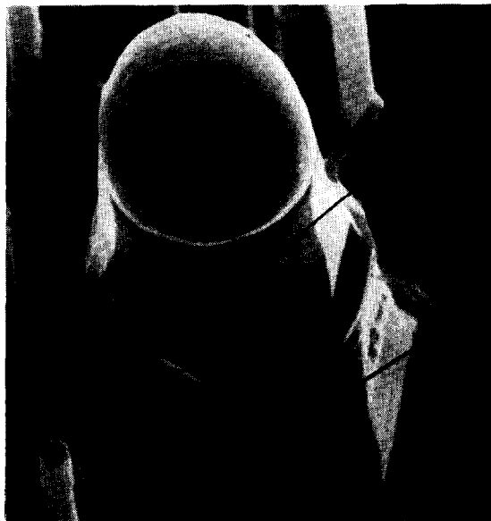
Fig. 5. Composite whisker "silicon+lanthanum hexaboride" on (111) silicon substrate.
