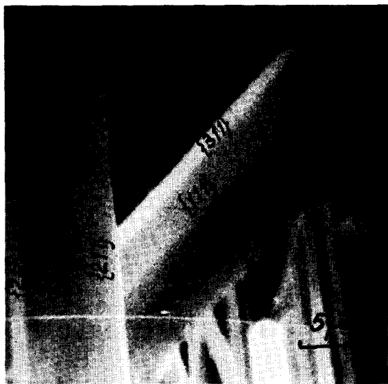
Fig. 2. Habitus of silicon whiskers grown in [111] and [1\bar{1}0] directions.
