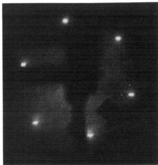
Fig. 4. (1 \times 1) LEED pattern of (000\bar{1})\text{ZnO} face after pretreatment according to fig. 3b.
