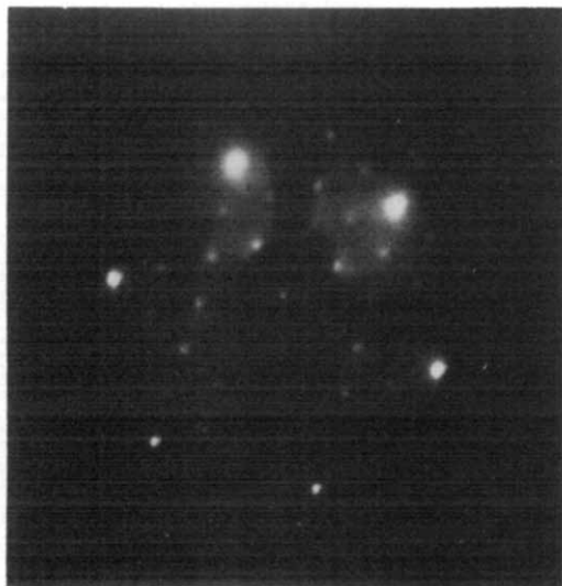
Fig. 6. (2\sqrt{3} \times 2\sqrt{3}) overlayer structure caused by potassium contamination on (0001̄)ZnO.
