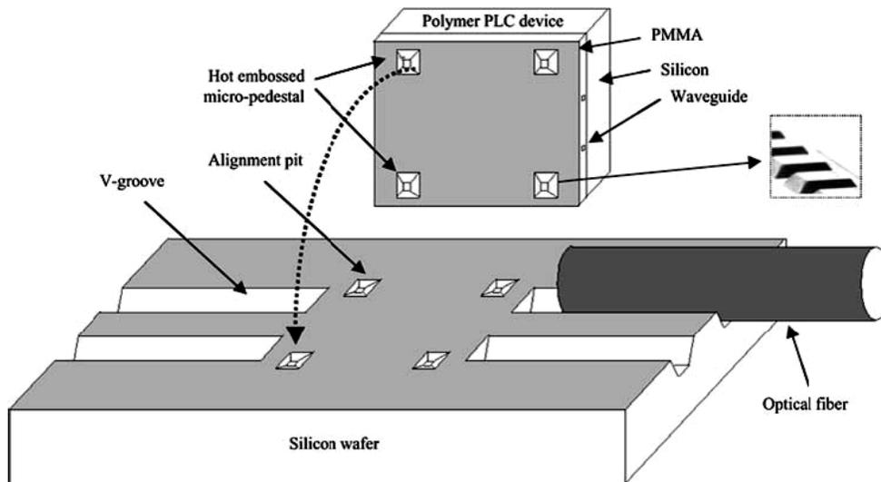
Fig. 9. Principles of the passive alignment of a hot embossed polymer PLC device [24]
