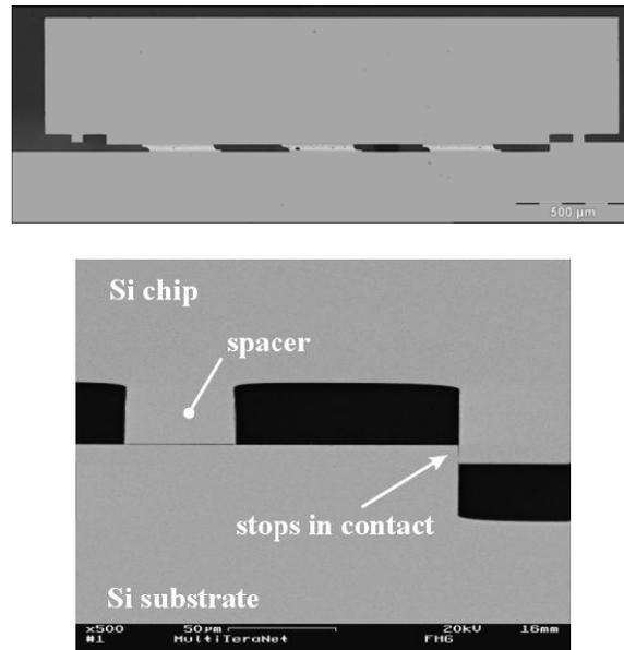
Fig. 2. Cross-sectional images to show how spacers and stops determine the final positions of the chip [7]
