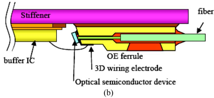
Fig. 8. Cross-sectional view of POST LSI package (a) and Cross-sectional view of optical module [23]
