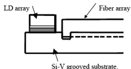
Fig. 15. Optical coupling scheme of transmitter [31]
