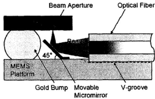
Fig. 10. A cross-sectional schematic view of laser to fiber coupling concept [25]
