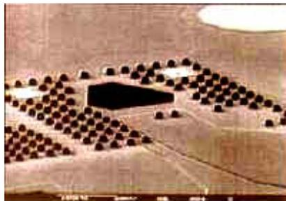
Fig. 1. SEM photo of the Indium bumps for VCSEL hybridization and hole etched for fiber placement [6]
