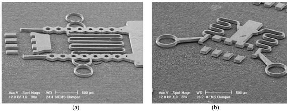
Fig. 11. SEM pictures: (a) Type-1 micro clammer structure. (b) Type-2 micro clammer structure
