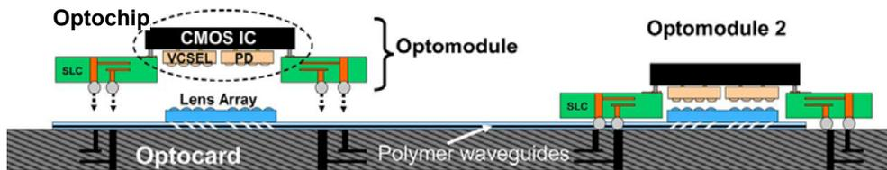
Fig. 4. Schematic of IBM Terabus package [9]
