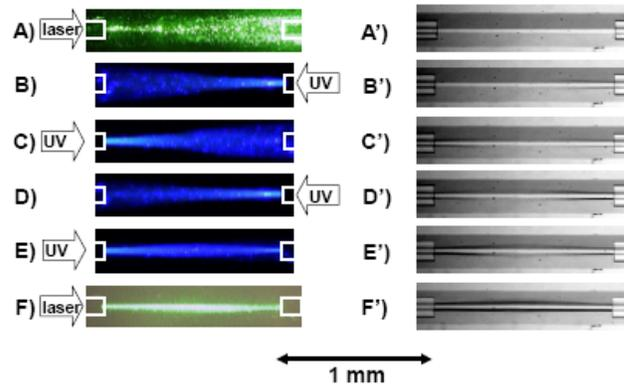
Fig. 6. Optical coupling of gapped MMFs using self-written waveguides (both-side exposure). The left is light guiding behavior. The light input directions are marked on each. The right is corresponding actual waveguides view. A: Green laser irradiation at initial state (the gap is filled with uncured resin). B, C, D, E: Step#1 - #4 of both-side exposure with UV intensity: 0.7 mW/cm<sup>2</sup>. F: Green laser irradiation after step#10
