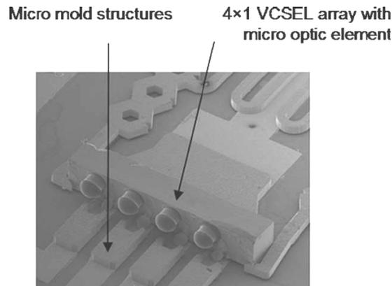
Fig. 12. A  $4 \times 1$  VCSEL array held in position by a type-1 micro clasper
