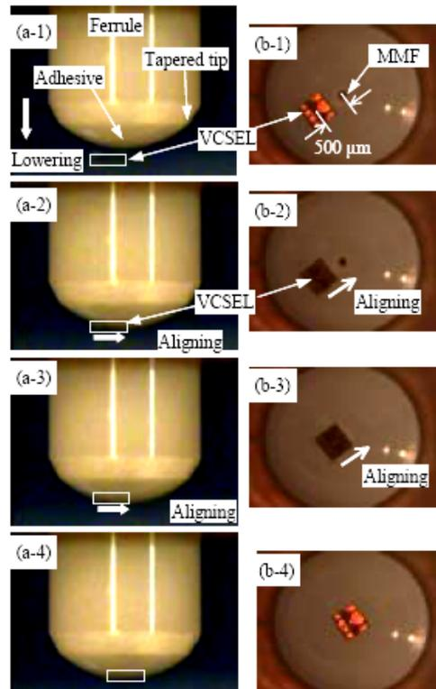
Fig.5. Process of self-aligning VCSEL to MMF: Photos a-1 to a-4 show the side views with the adhesive and VCSEL while b-1 to b-4 show the bottom view [12]
