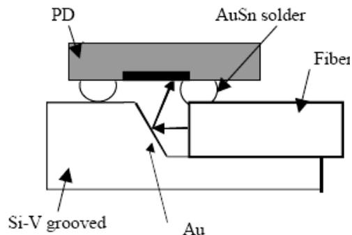
Fig. 16. Optical coupling scheme of receive [31]
