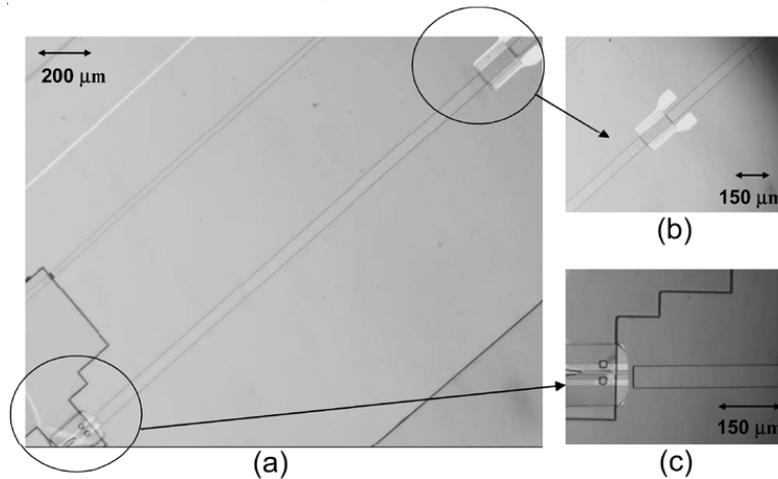
Fig. 14. Fabricated point to point optical interconnection system using a thin-film laser and a thin-film I-MSM PD [30]
