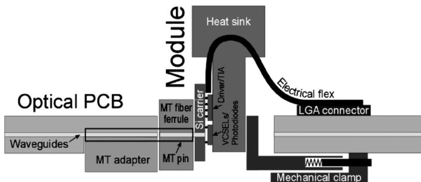
Fig. 8. Schematic of the optical module passively aligned onto the embedded waveguides [22]
