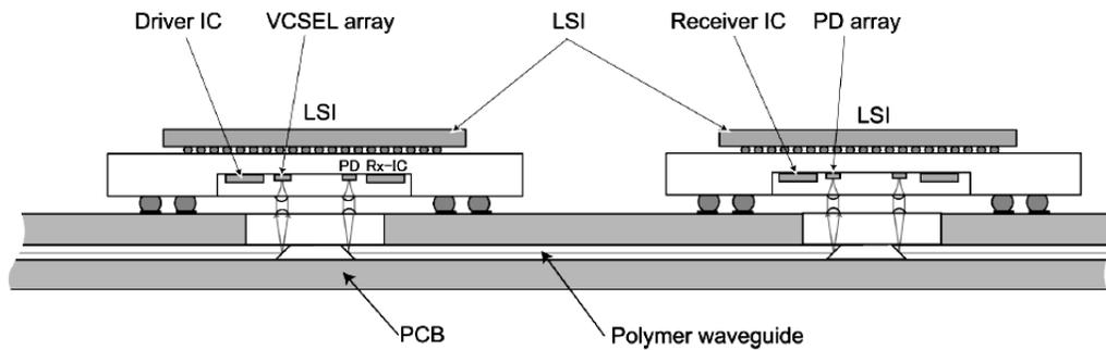
Fig. 3. Schematic of on-PCB optical interconnection based on the OptoBump interface [8]
