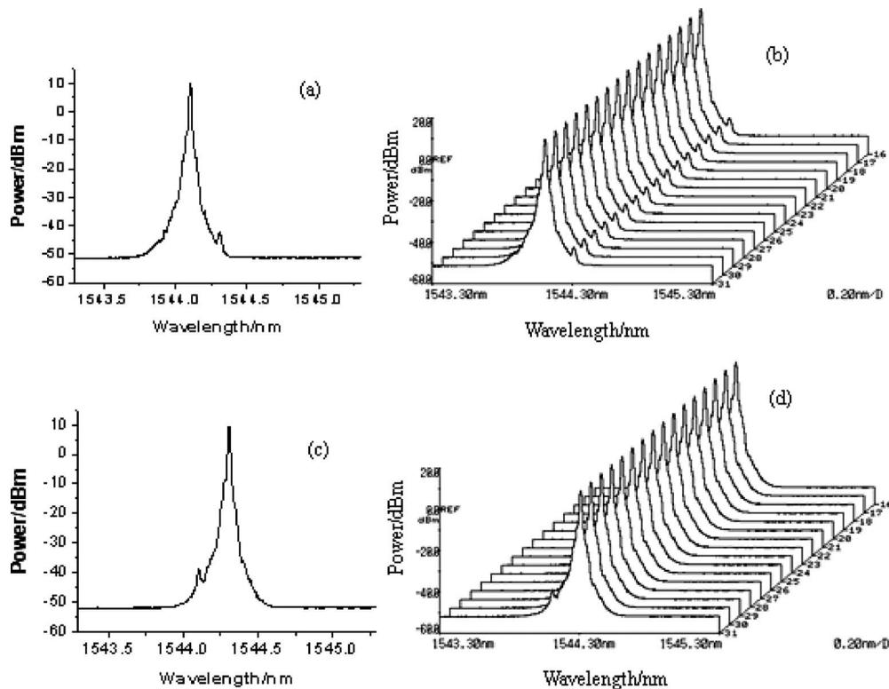
Fig. 4 Single-wavelength operation of the laser at ~110 mW pumped.
