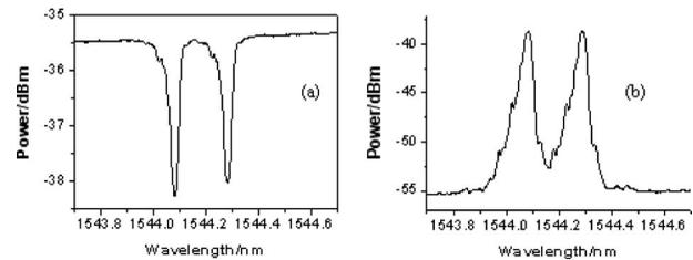
Fig. 2 The transmission spectra (a) and reflection spectra (b) of PMFBG.
