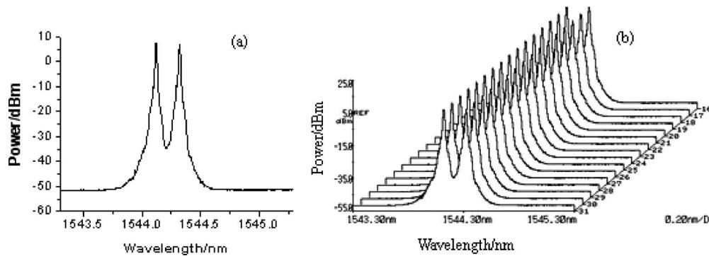
Fig. 3 Dual-wavelength operation of the laser at ~110 mW pumped.
