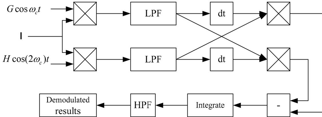
Fig.1 The frame of the PGC technique
