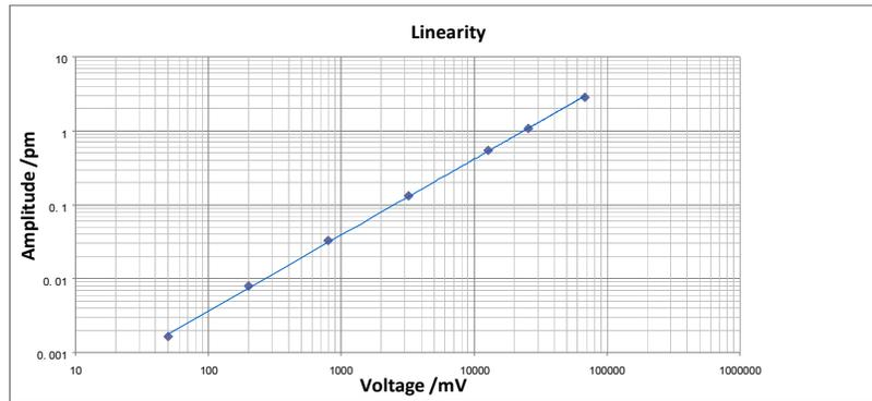
Fig.9 The linearity at the frequency of 100Hz
