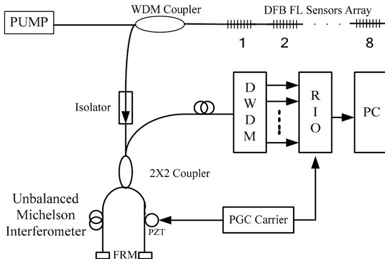
Fig.2 Schematic diagram of the proposed Eight-elements DFB FL sensors array system
