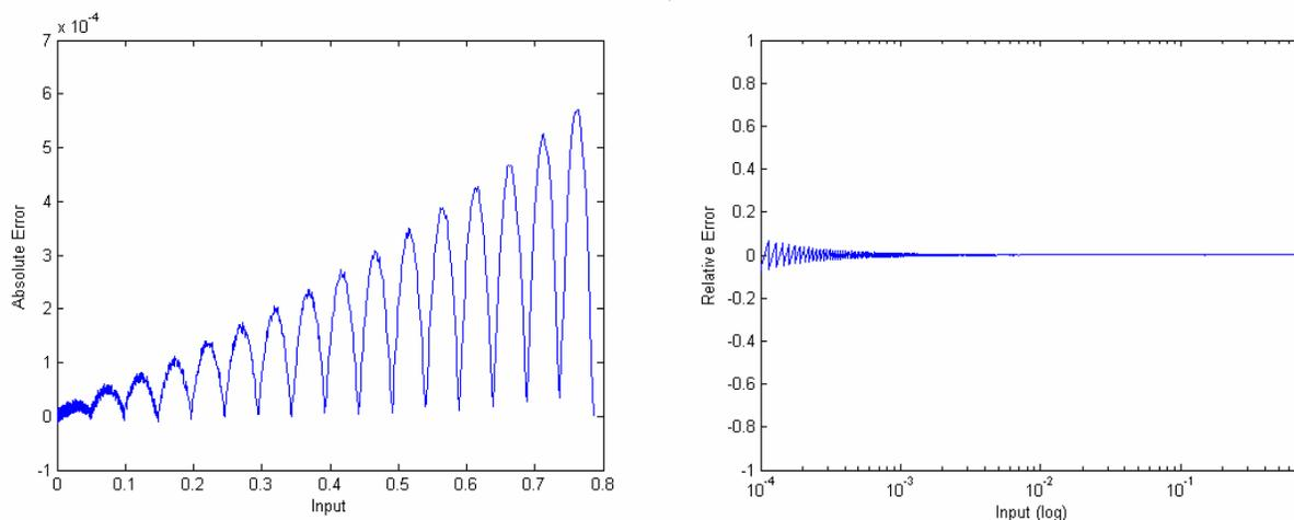
Fig. 3: The error of the Table-Lookup arctangent method;
