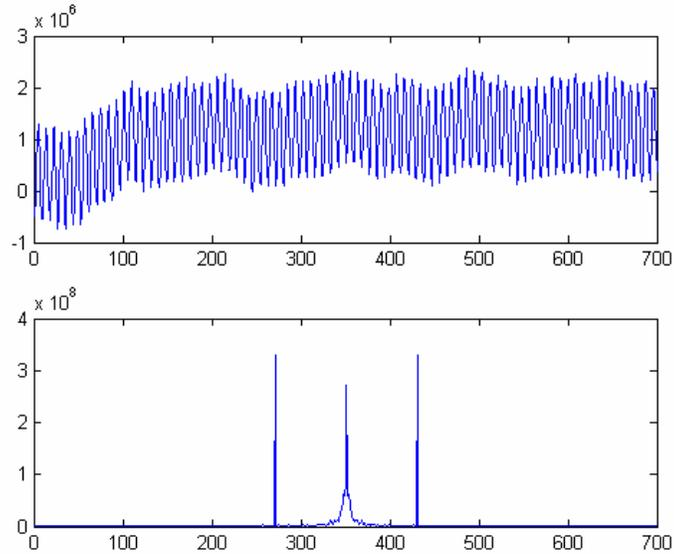
Fig. 9: the influence of the light power to the arctangent PGC approach.
