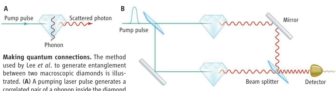
**Making quantum connections.** The method used by Lee *et al.* to generate entanglement between two macroscopic diamonds is illustrated. (A) A pumping laser pulse generates a correlated pair of a phonon inside the diamond as well as a scattered photon. (B) The scattered photons from two diamonds are brought together for interference and detection. When one photon is detected, the two diamonds coherently share a phonon. Thus, the quantum state created has the hallmarks of quantum entanglement.
