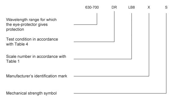
If several marks apply to a laser radiation eye-protector, all these marks shall be applied, or alternatively the manufacturer's identification mark, the certification mark and the mechanical strength symbol shall be specified only once; the other identification elements shall be separated by a +.
