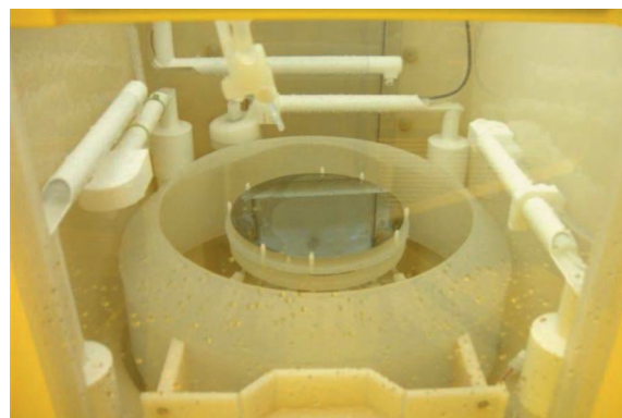
Figure 2. The single wafer spin processor chamber.
