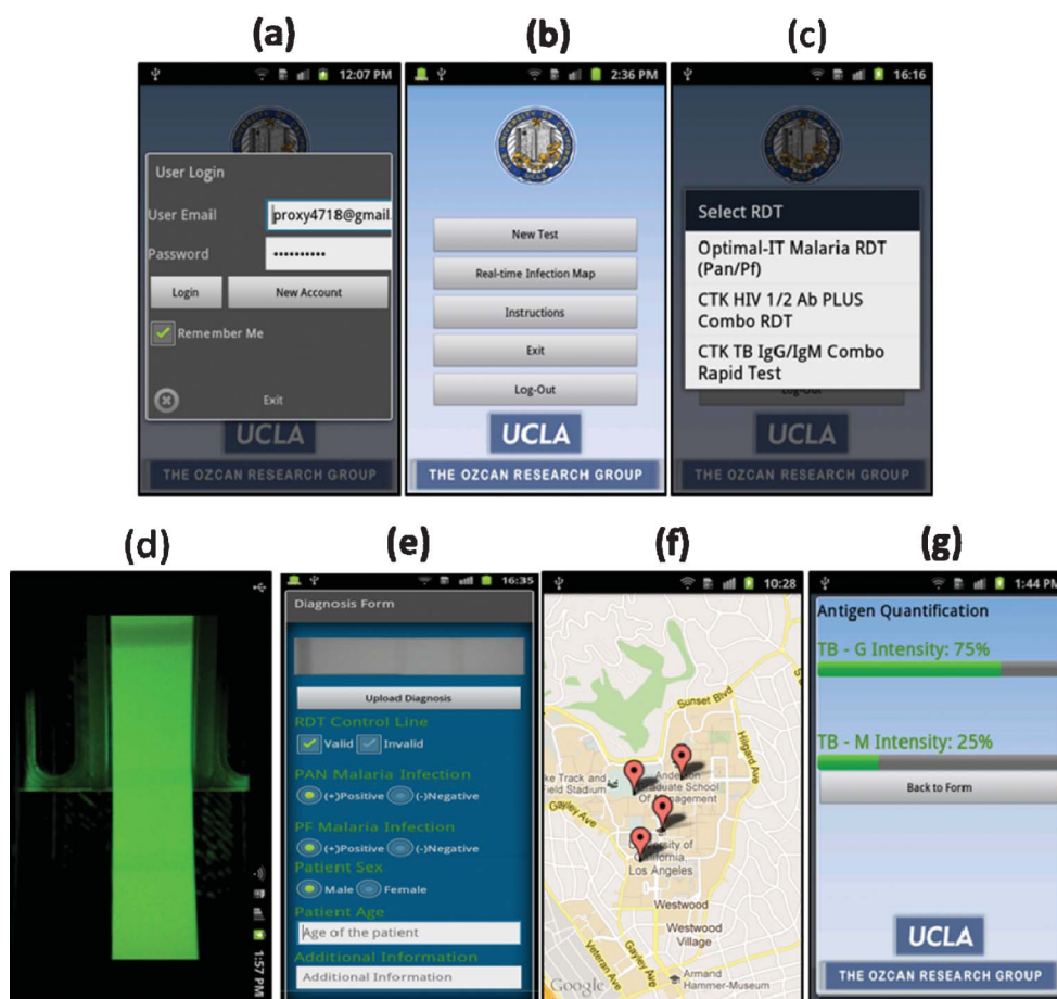
Fig. 2 (a) User Login screen of the Android application running on the cell phone device that is shown in Fig. 1. (b) Main menu of the application is shown. (c) Once user selects to image a new RDT, a pull-down menu of the pre-configured RDTs pops up. (d) Upon the selection of RDT type and illumination scheme (reflection or transmission), the application displays a raw image of the test. User can then touch the screen to capture, digitally process and evaluate the test results. (e) RDT Evaluation menu displays test results including validity of the test (valid/invalid), decision of infection (positive/negative) for each test type, as well as other information that the user can manually enter. The same application then uploads this test result to our database/server (f) that is protected by password. In case wireless connection is not available, it saves the results to the cellphone memory to be transmitted later. (g) Our application can also quantify the relative antigen density for each test line. To perform this antigen density measurement, RDT application needs to be calibrated by imaging a blank unfunctionalized test (for minimum color intensity) and a saturated test (for maximum color intensity) that is functionalized using positive control antigens. Then the application returns the ratio of antigen density compared to reference values per test line. Note that for each RDT type, this calibration needs to be performed only once.
