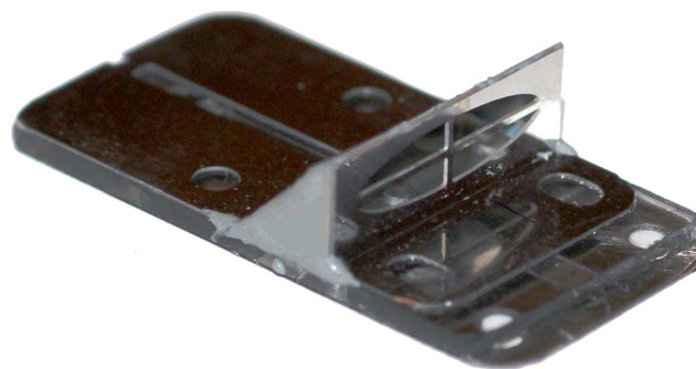
Fig. 6 Photograph of device IV, 30 mm long and 15 mm wide, with a raised intake funnel, 5 mm high. The intake has a coarse grid to prohibit larger particles from entering and clogging up the intake. Behind the intake, an elongated opening in the cover sheet enables viewing of the microfluidic channel beneath. At the end of this window is the outlet of the microfluidic channel.
