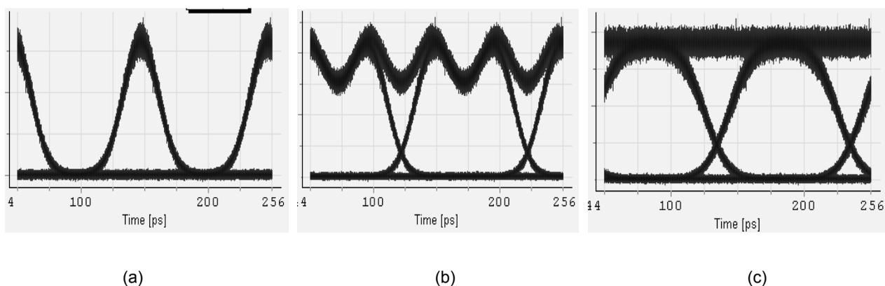
Fig. 4 Eye diagrams for the RZ to NRZ conversion (a) original RZ signal (b) preprocessed signal (c) converted NRZ signal
