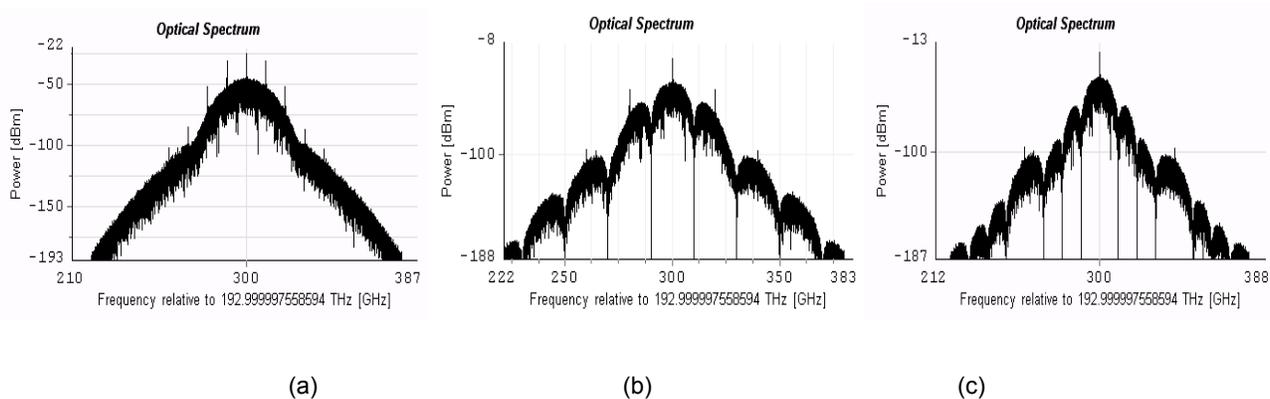
Fig. 3 Spectral evolutions for one of the multi-channel signals (a) RZ signal (b) Preprocessed signal after the first DI (c) converted NRZ signal
