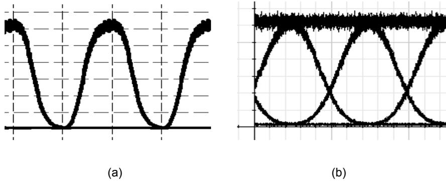
Fig. 5 Eye diagrams for the RZ to NRZ conversion with 50% duty cycle (a) original RZ signal (b) converted NRZ signal
