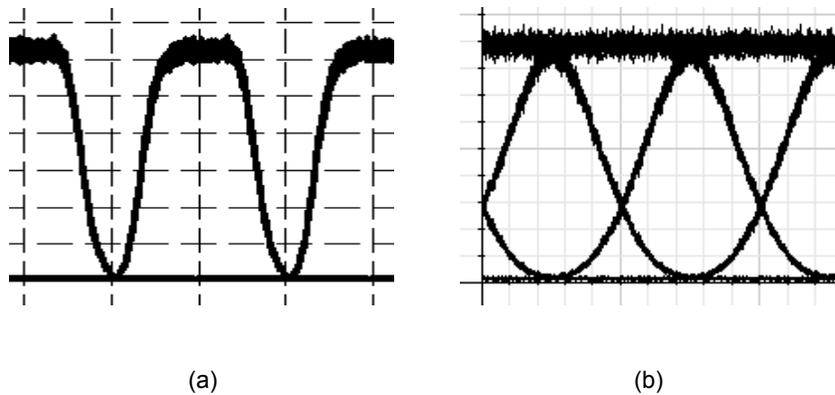
Fig. 6 Eye diagrams for the RZ to NRZ conversion with 66% duty cycle (a) original RZ signal (b) converted NRZ signal
