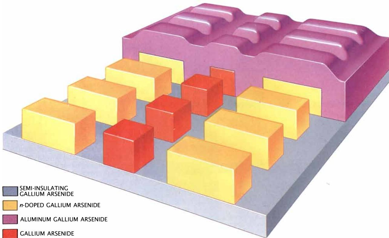
QUANTUM CHIP has features 100 times smaller than those of standard chip components. Current flows from one negatively doped (*n*-doped) gallium arsenide block to another through a layer of aluminum gallium arsenide, a gallium arsenide cube and then another aluminum gallium arsenide layer. Because of cer-
