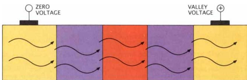
TUNNELING ELECTRONS (arrows) resonate in a gallium arsenide quantum well (red) when a positive bias called the resonant voltage is applied to one of the contacts (top). The electron waves bounce back and forth inside the well, enhancing the current to give rise to the peak on the graph at the top of this page. At the valley voltage (bottom) little tunneling or resonance takes place, consequently the current dips dramatically.
