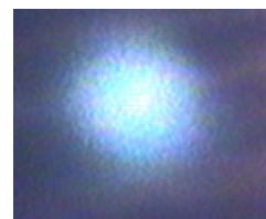
FIGURE 3: The beam spot of the Nd:YVO 4 fluorescence beam. Mag. 1X
