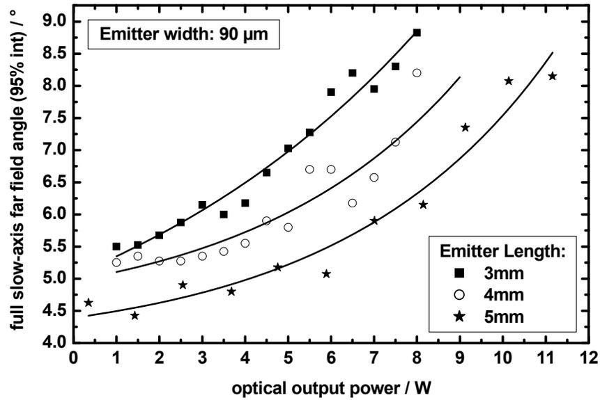
Figure 2: Length dependence of the full slow-axis far field angle (measured with 95% integral method) for device geometries of 3mm, 4mm and 5mm emitter-length and 90 $\mu$ m emitter-width. Due to better heat dissipation the device with 5mm length reaches the lowest slow-axis far field angles below around 8° up to output powers of nearly 10W. (measurement conditions: CuW-Submount onto C-Mount, cw-mode, 20°C)
