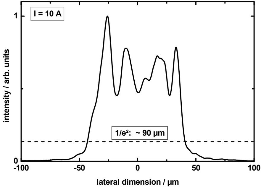
Figure 4: Typical near field of a broad area laser with 5 mm resonator length, mounted on C-Mount with a CuW-Submount. Up to 10A the near field width at a level of  $1/e^2$  stays well below  $100\mu\text{m}$ . Together with a low value for the slow-axis divergence angle this leads to a high brightness, doubled compared to commercial available BA-Lasers. The measurement was done in cw mode at a heat sink temperature of 20°C.
