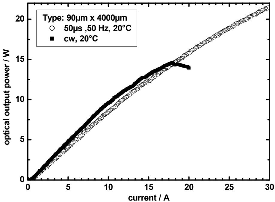
Figure 6: Optical output power against operation-current of a broad area laser with 4 mm resonator length in cw mode limited to  $> 14 \text{ W}$  by thermal roll over due to mounting (solid) and in pulsed mode at pulse length of 50μs and a repetition
