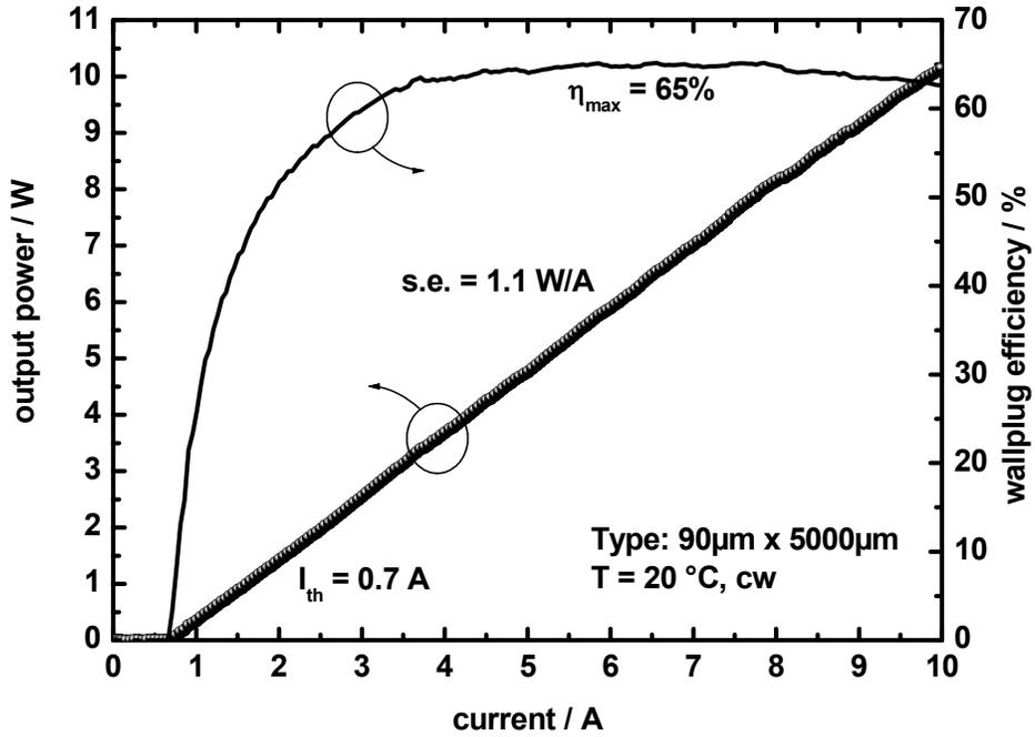
Figure 1: Optical output power against operation-current (solid dots) and wall-plug efficiency (line) of a broad area laser with 5 mm resonator length in cw mode at a heat sink temperature of 20°C. An output power of 10W has been achieved at 9.8A. A wall-plug efficiency of 65% has been measured. To our knowledge, for a 5mm long device, this is the highest wall-plug efficiency reported so far.
