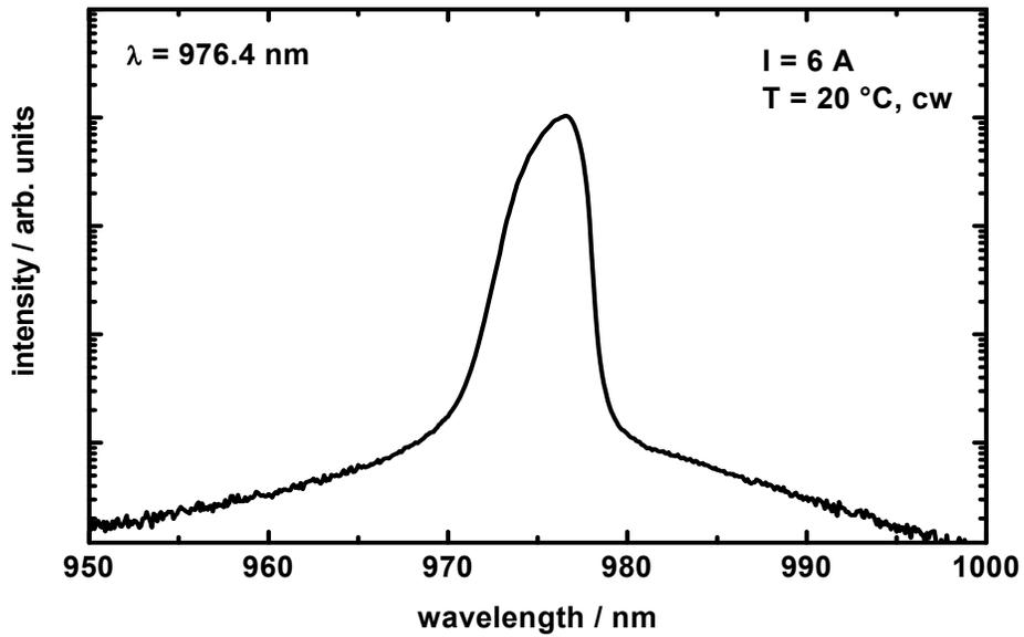
Figure 5: Typical spectrum of a broad area laser with 4 mm resonator length in cw mode at a heat sink temperature of 20°C. At a current of 6A a center-wavelength around 976 nm is reached, which is well suitable for pumping of Yb-doped fibers.
