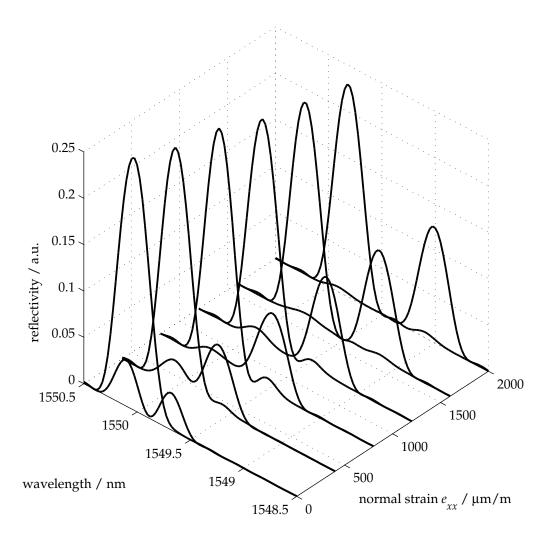
**Figure 4.** Six simulations with increasing normal strain and a fixed shear strain of  $e_{xy} = 2000 \,\mu\text{m/m}$ . For low normal strains, the reflection peaks are only separated by the birefringence of the fiber and polarization mode coupling is high, leading to a strong second peak in the *s*-mode reflection spectrum. For higher normal strain loads, the peaks separate further and polarization mode coupling is reduced.
