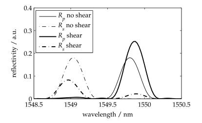
**Figure 3.** Result of the simulation using a normal strain  $e_{xx} = 2000 \,\mu\text{m/m}$  and  $e_{yy} = -me_{xx}$ , m = 0.2. The shear strain is neglected in the thin lined result and set to 2000  $\mu\text{m/m}$  for the simulation with shear strain. The results without shear strain show the expected shift of the spectral response, without changing the shape of the spectrum. With shear strain, the polarization modes couple and the reflection spectra are changed in shape.
