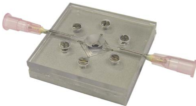
Figure 38 (online color at: www.lpr-journal.org ) The microfluidic sensing cell [16].
